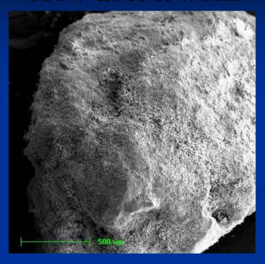
Zeolites are hydrated aluminosilicates of alkali or alkaline-earth metals (Na, K, Mg, Ca, Sr, Ba)
