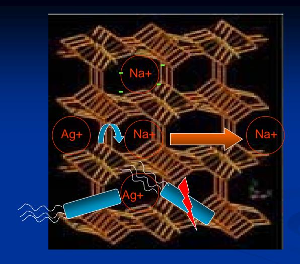
Ag strongly binded into the crystalline building of the zeolite can exert a powerful bactericidal effect by complexing the sulphydrylic groups of the bacterial membrane proteins causing the denaturization and irreversible destruction of the microbial cell membrane
